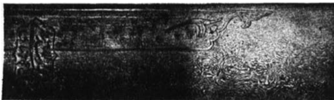
Figure 15.38 Section of a blade of Damascus steel showing the characteristic damask or ‘watering’ pattern.
