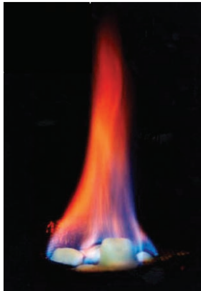
Figure 7.1 ‘Burning snowballs’ of methane clathrate hydrate (image courtesy of the US Geological Survey).
