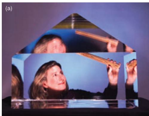
Figure 8.8 Very large crystals such as this sample of KDP ( \text{KH}_2\text{PO}_4 ) used for laser frequency doubling are produced by careful nucleation control at the metastable boundary between an unsaturated and supersaturated solution (image courtesy of the Lawrence Livermore National Laboratory).
